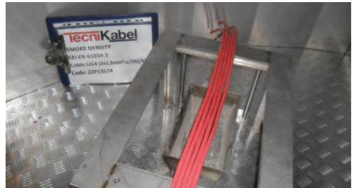
**Measurement of smoke density of cables burning under defined conditions**
