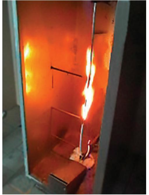
**Test for vertical flame propagation for a single insulated wire or cable.**
